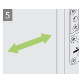
Seal contact pressure: push the hinge in the required direction (+/-1 mm); the teeth will hold the door leaf at the correct height. Fully tighten the adjusting screws in the frame part of the hinge.
