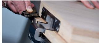
Once the hinge has been screwed into the wing, the wing seal is fitted. This is accommodated within the hinge with the aid of the sealing groove and continues in the joint area in the form of a seal specific to the hinge.
