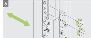
Joint clearance at the side: turn the adjusting spindles in the frame part of the **MASTERBAND** FX2 120 3-D CS to achieve exact positioning of the door leaf. The adjustment range is +/- 3 mm.
